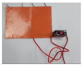
Silicone rubber heater is made of silicone rubber and alass fiber cloth compounded Silicone sheet, rubber heater has good flexibility, can be associated with an object to be heated is close contact; the heating elements of nickel alloy foil processing form, more uniform heating. In this way, we can let the heat transfer to any desired place.
