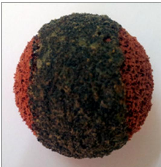
**Ring Carborundum Sponge Balls** also called as abrasive balls are the sponge balls coated with the ring of hard carborundum material. The carborundum is very hard; it can abrade hard deposits on the inner side of the tubes. So if on your condenser tube there is something stuck on the inner surface and very difficult to remove, the carborundum coated ball is the best choice.
